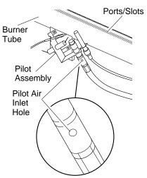
Figure 42 - Pilot Inlet Air Hole
